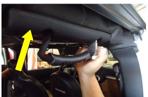
STEP 4: SCREW THE GRAB HANDLE INTO THE SLOTS USING A 10 MM SOCKET.
