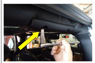
STEP 3: WHEN INSTALLING THE REAR JK GRAB HANDLES, REMOVE THE (2) SCREWS USING A 10 MM SOCKET.
