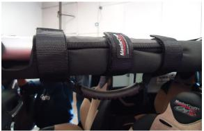
STEP 2: RUN THE STRAPS THROUGH THE BUCKLES AND PULL EACH ONE TIGHT AS YOU VELCRO IT IN PLACE.
